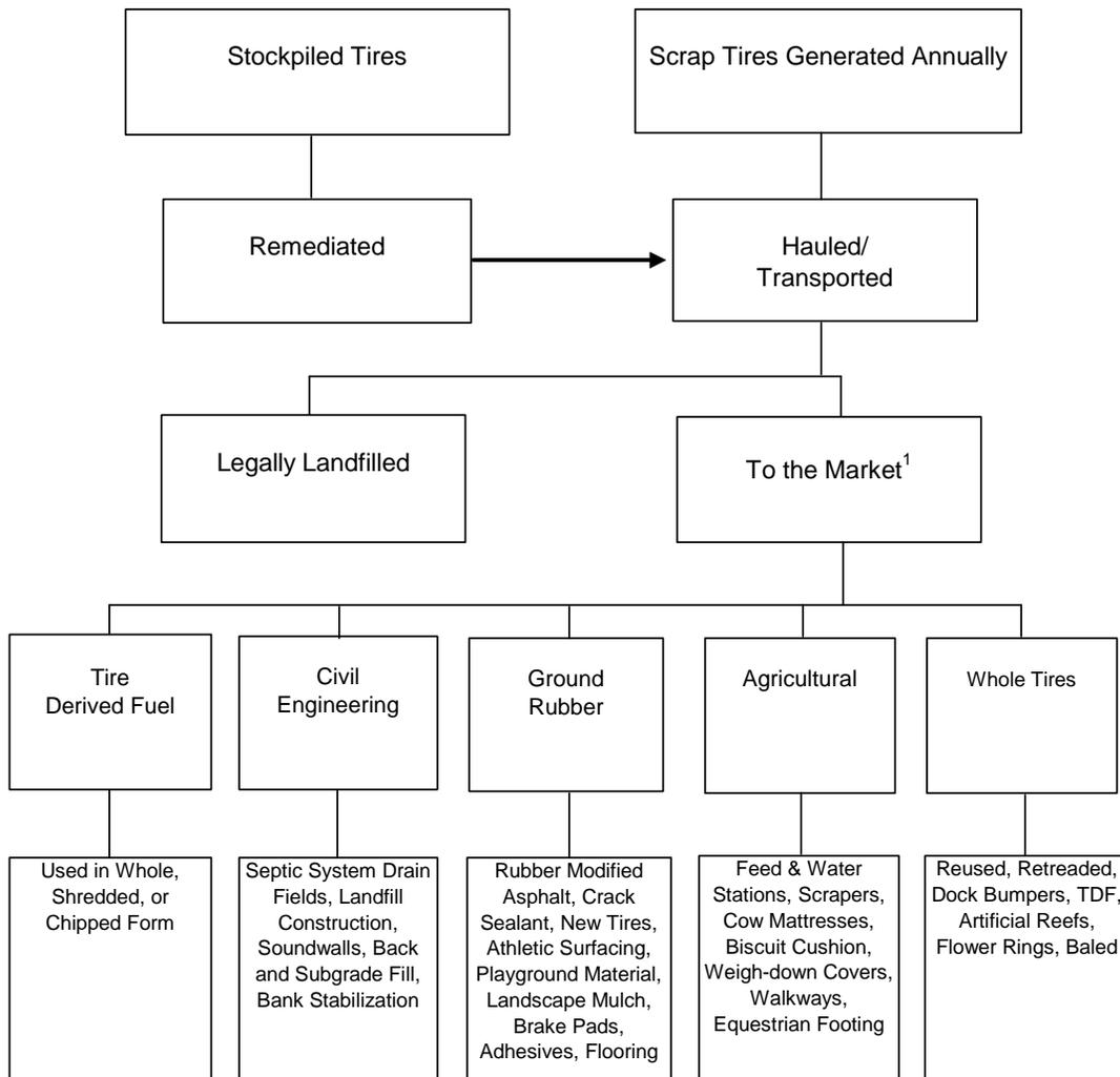
1. Tire types such as passenger, truck, industrial, off-road, bias ply, etc., can not all be utilized to create the same products.
